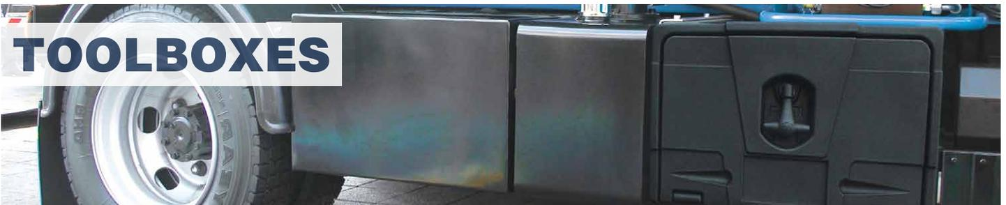
Toolboxes are best fixed using our support bracketry which ensures that even heavy loads do not cause damage to the box. Under European law our toolboxes can be used in place of a section of a side guard rail and several companies fit tool boxes to the vehicle to act as a side guard rail. Toolboxes are exempt from the side guard rail legislation in Europe (please check yourself for any regional or recent changes to this) and do not have to pass the impact test.
